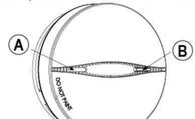
A. Buzzer hole B. Test / Mute button & LEDs
